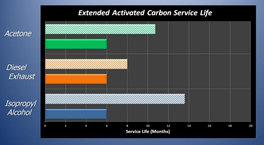
*Note: test results from 3rd party laboratory. striped bars with oxidant, solid bars without oxidant*
