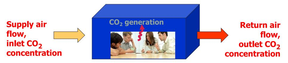
Also can consider as: CO<sub>2</sub> removal = Outdoor air flow x [outlet-inlet] CO<sub>2</sub> concentration
